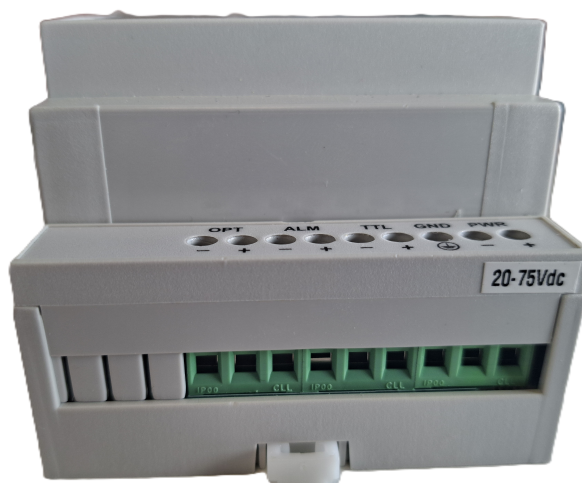
Figure 5-1. Power Supply Voltage Input Label Above PWR Screw Clamps
