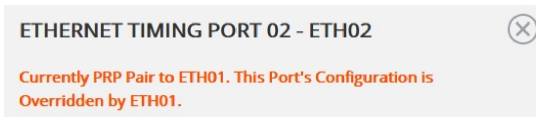
Figure 9-54. Warning on PRP LAN B Setting
