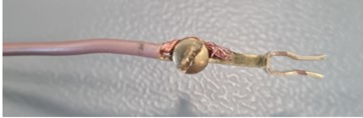
Figure 15-2. Screw Holding Copper in Place
